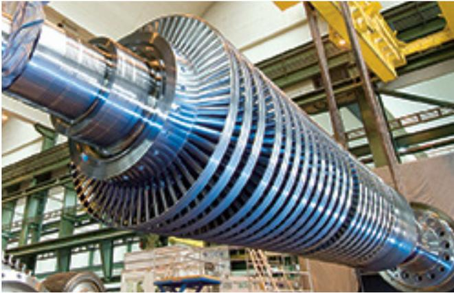
**S**tream turbines go around. Since their invention in 1884, they have made much of the industrial world go around, as well. Sometimes referred to as the perfect engine, steam turbines rapidly replaced the steam engine due to greater efficiency at converting heat into motion and motion into power. Their rotary action also became the primary power source for driving generators to create electricity.
